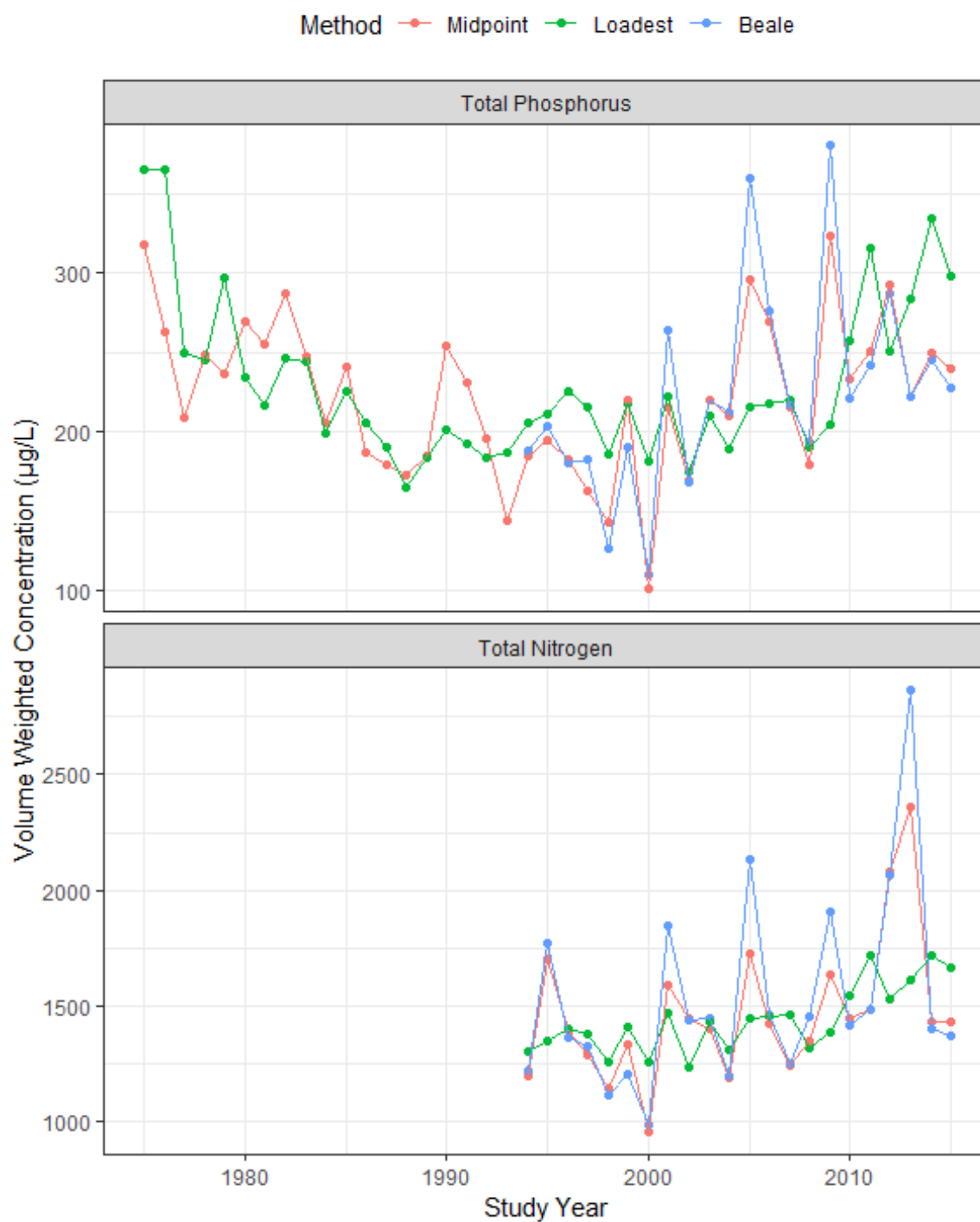
Figure 93: Volume-weighted nutrient concentrations calculated annually for the Qu'Appelle River at Welby. Volume-weighted concentrations were calculated using monthly sampling data from the Prairie Provinces Water Board. Results from three calculation methods are presented. Concentrations were calculated using a year from March 01 - February 28/29 to match our study.
